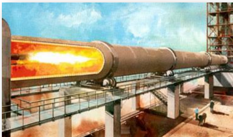
Rys. 1. Piec do wypalania klinkieru http://www.machineryandequipment.com/featured/kilns.html
